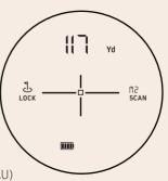
UTILISEZ LE MODE "PIN SEEKER" (POUR TROUVER L'OBJET VERTICAL LE PLUS PROCHE) POUR MESURER LA DISTANCE À UN DRAPEAU SUR UN GREEN AVEC DES ARBRES EN ARRIÈRE-PLAN, AINSI QUE POUR MESURER DES CIBLES QUI SE CHEVAUCHENT. IL EST ÉGALEMENT BON DE L'UTILISER PAR TEMPS VENTEUX. LA FONCTION DE VERROUILLAGE VOUS PERMET D'EFFECTUER VOTRE TIR EN TOUTE CONFIANCE
