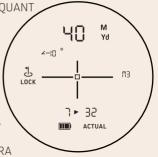
UTILISEZ LE "MODE PENTE" POUR DÉTERMINER LA DISTANCE DE L'OBJET LE PLUS PROCHE. CE MODE EST ÉGALEMENT CONNU SOUS LE NOM DE "FONCTION DE PRIORITÉ AUX OBJETS LES PLUS PROCHES".
