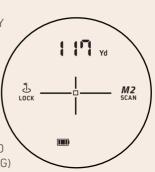
USE **PIN SEEKER MODE** TO FIND THE CLOSEST VERTICAL OBJECT SUCH AS THE DISTANCE TO A FLAGSTICK ON A GREEN WITH WOODS IN THE BACK-GROUND; AS WELL AS WHEN MEASURING OVERLAPPING TARGETS.
